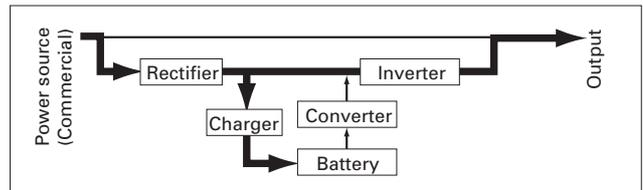
Figure 3 Power supply quality priority mode power supply circuit
