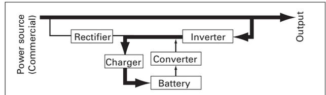
Figure 4 Efficiency priority mode power supply circuit
