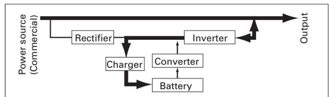
Figure 5 Active filter mode power supply circuit
