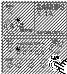
Press 3~4 seconds and release it when the buzzer rings "beep, beep".
